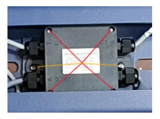
After removing the cover, a luster terminal is revealed. The defective cable can be disconnected here, and the new one connected in the same way.
